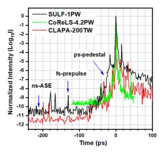
**Figure 4.** The temporal profiles of three ultraintense femtosecond laser pulses from the SULF, CoReLS, and CLAPA facilities, respectively.
