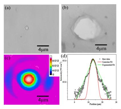
Figure 1. The damage morphologies of a formvar target under laser irradiation at the intensity of (a)  $6 \times 10^{12}$  W/cm<sup>2</sup> and (b)  $1.1 \times 10^{13}$  W/cm<sup>2</sup>. (c) The intensity distribution around the focal spot. (d) A line out of the laser intensity across the focal spot (scattered black circle), the corresponding Gaussian fit (red line), and the exponential fit (green line) of the raw data.
