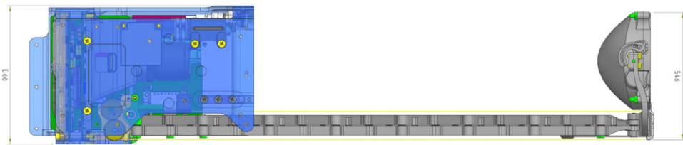
Figure 4. MANTIS payload fully deployed with convex-surfaced mirror facing satellite for self-imaging (side view).
