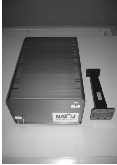
Figure 1. Ambient temperature 6.7 GHz receiver, T_{rx} = 60 K. Designed and built in Nobeyama Radio Observatory of NAOJ
