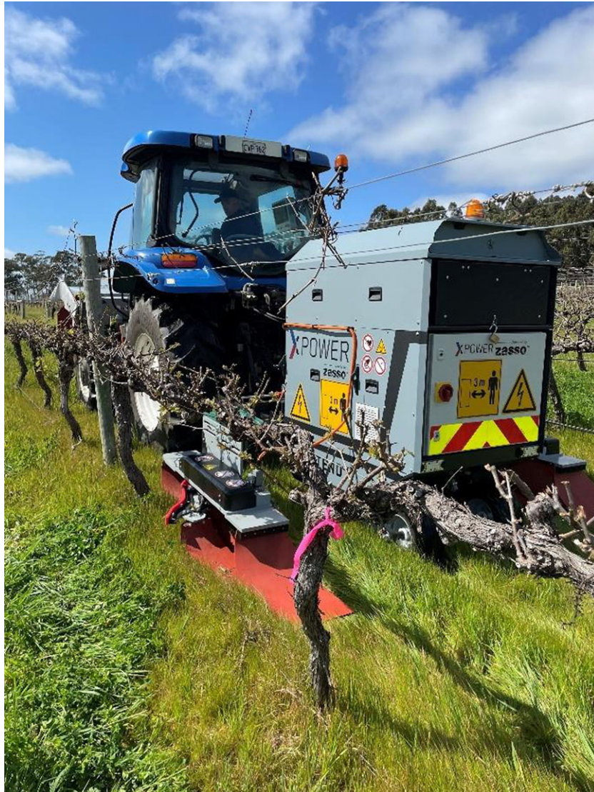
Figure 1. Tractor with an XPower electric weed control machine (Zasso™). The power supply unit is on the rear linkage, and the XPS applicators are on each side of the supply unit, with front and rear static electrode arrays and center electrode array on a retractable arm. The electrode arrays are shielded by red rubber mats to contain sparks.
