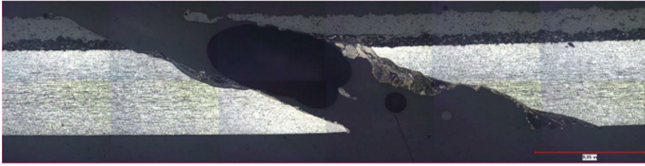
Figure 7. Recast Layer Coupon TL21-196-1 (500X).
