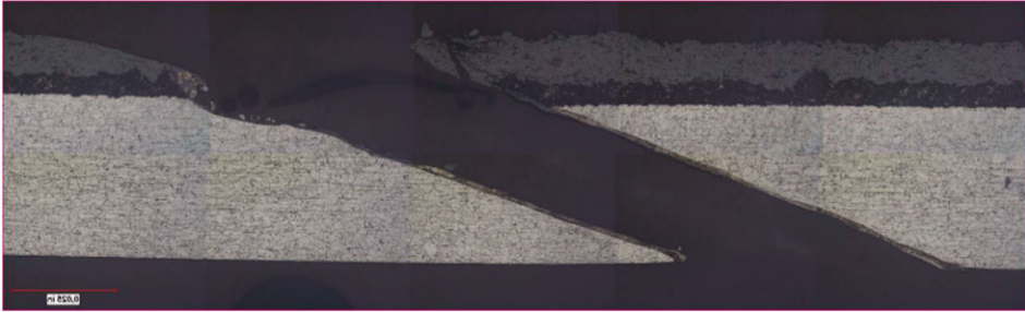
Figure 17. Recast Layer Coupon TL22-055-2 (500X).
