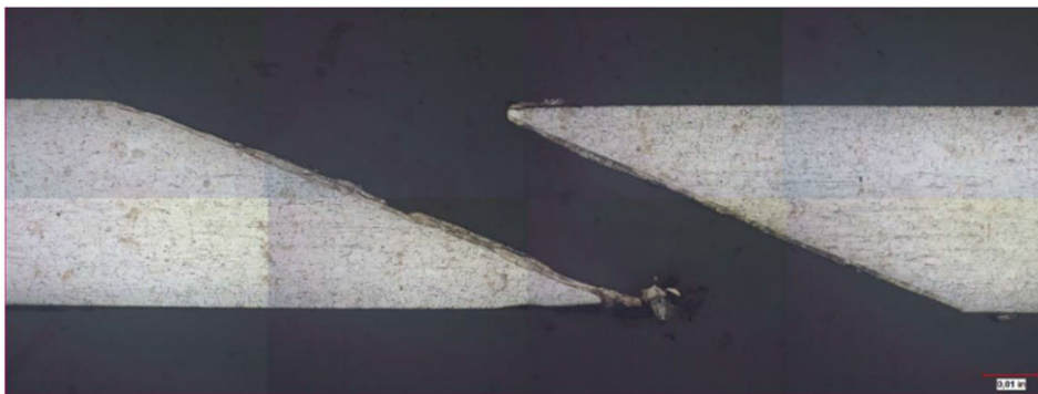
Figure 21. Recast Layer Coupon TL22-073-1 (without TBC, 500X).
