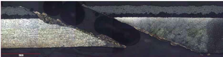
Figure 12. Recast Layer Coupon TL21-196-6 (500X).
