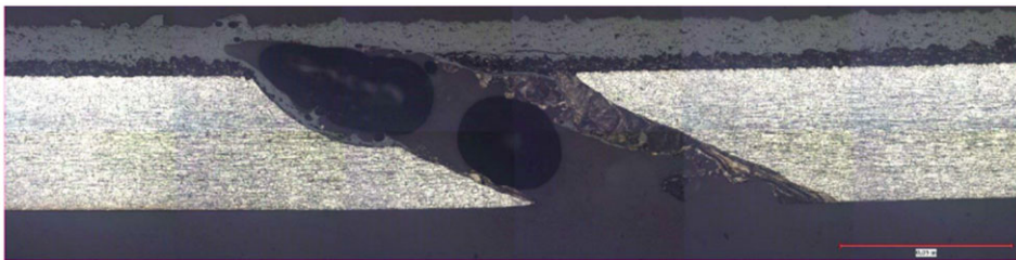
Figure 8. Recast Layer Coupon TL21-196-2 (500X).
