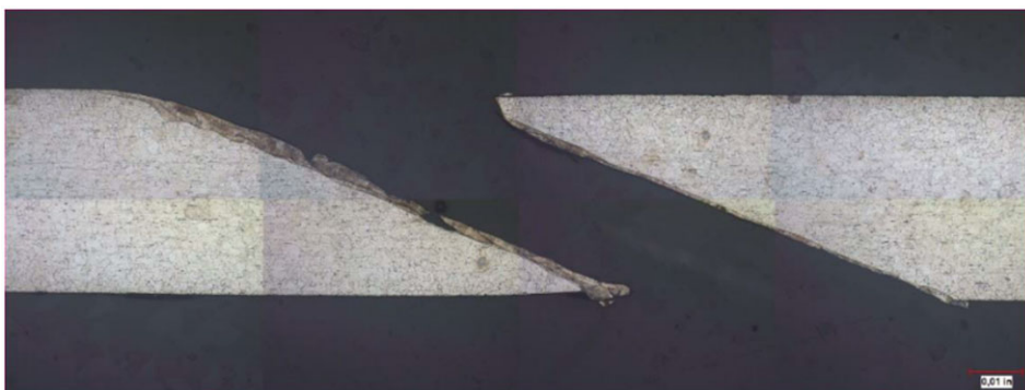
Figure 22. Recast Layer Coupon TL22-073-2 (without TBC, 500X).
