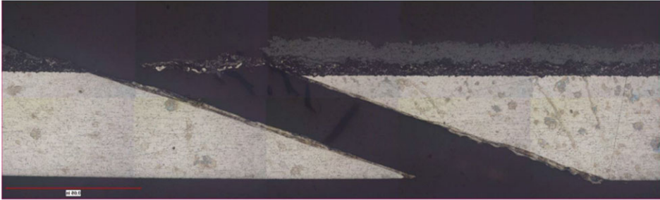
Figure 14. Recast Layer Coupon TL22-021-1 (500X).
