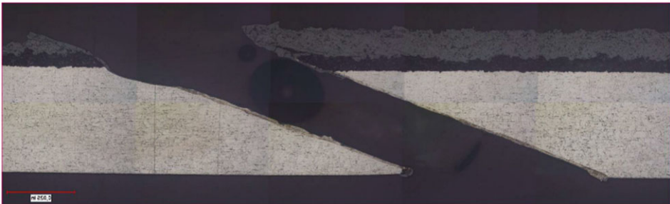
Figure 18. Recast Layer Coupon TL22-055-3 (500X).
