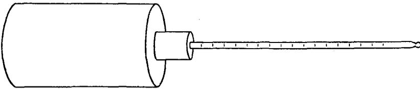
Fig. 1. Paint testing flask.
