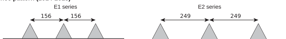
Fig. 4. Cross profiles of artificial bumps on which snow accumulated. (a) First version of the experiment in 2012–2013 with wooden battens with two periodic spacings. (b) Second version run in 2014–2015 with metal triangular profiles of various sizes on plywood tables. (c) Two series of E-type profiles were used to assess interference effects based on bump separation distances. All dimensions are in millimeters.
