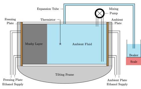
Figure 2. A two-dimensional schematic of the experiment apparatus.
