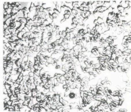
Fig.8. Photograph of snow particles immersed in kerosene (after 100 hr).
