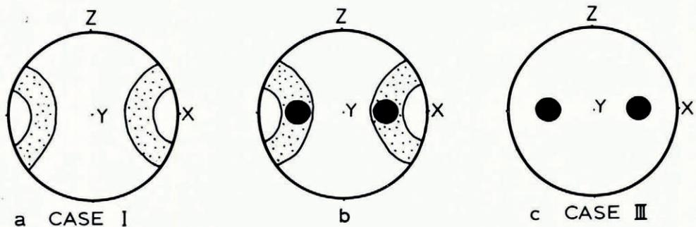
Fig. 7. a. Case I of the fabrics predicted by Brace;  $X : Y : Z = -\sigma' : +\sigma'/2 : +\sigma'/2$ .
