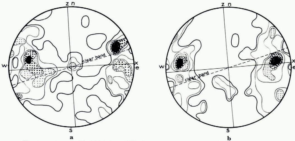
Fig. 5. a. 224  $c$ -axes of ice (CF<sub>2</sub>) from grid F. Contours 1-2-3-4-5  $<$ %; maximum 5% per 1% area. Grain-size: 1.1 grains/cm<sup>2</sup>.
