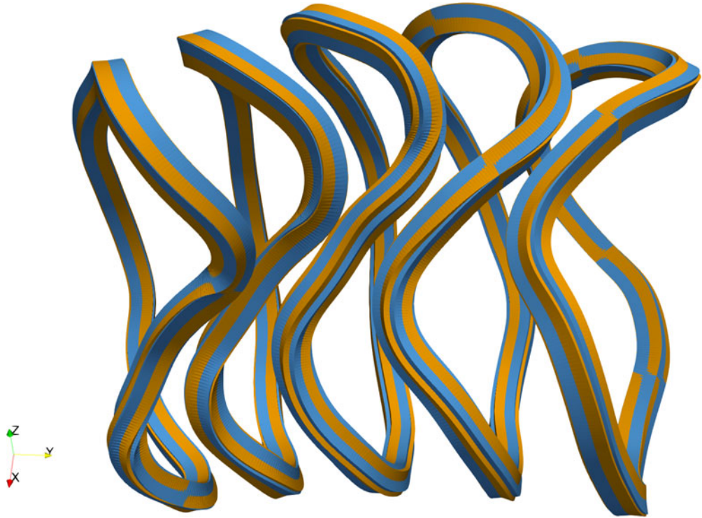
FIGURE 13. Winding packs (without casing) are displayed for the five independent coils with the pure centroid orientation (blue) and the optimised one (orange). While subtle, the difference is visible, especially when focusing on the third coil.
