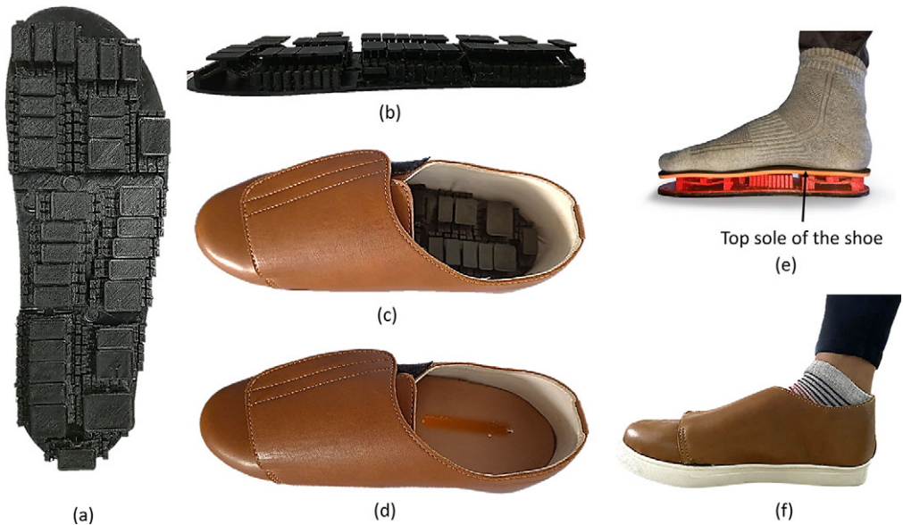
Figure 12. 3D-printed prototype of self-offloading insole and customized footwear: (a) top view of the insole, (b) side view of the insole, (c) footwear with the self-offloading insole (d) footwear with the self-offloading insole underneath the top sole, (e) 3D-printed in-sole with two layers of soft sole on it to provide cushioning effect, and (f) one of the volunteers wearing the self-offloading footwear.
