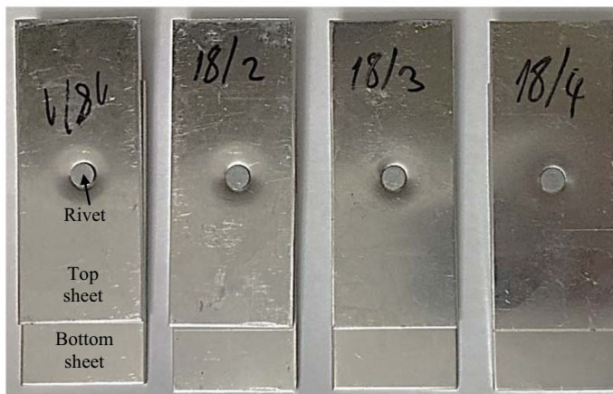
Figure 11. Samples no. 18-1, 18-2, 18-3 and 18-4 prepared for tensile-shearing.
