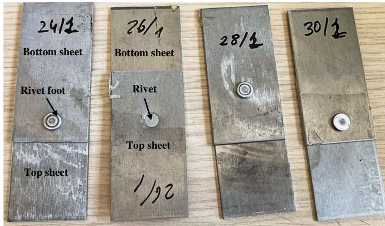
Figure 12. Samples no. 24-1, 26-1, 28-1 and 30-1 prepared for tensile-shearing.
