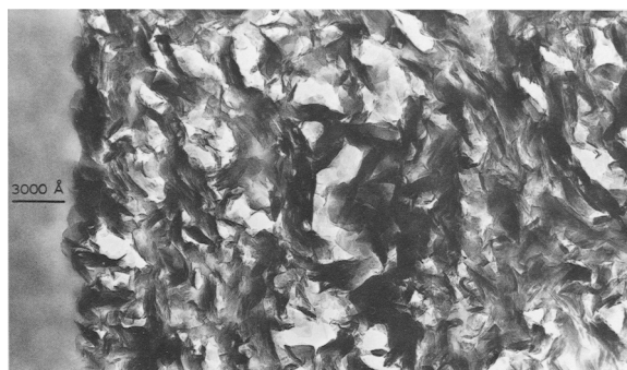
Figure 5. Transmission electron micrograph illustrating fabric of specimen of South Carolina vemiculitic material. Plane of "preferred orientation" is perpendicular to plane of micrograph and parallel to specimen-resin contact, evident on left side of micrograph.
