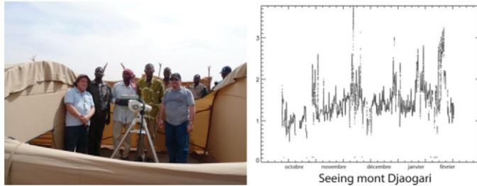
**Figure 4.** (left) Seeing monitor camera. (right) Seeing (image size) for the first 125 nights.
