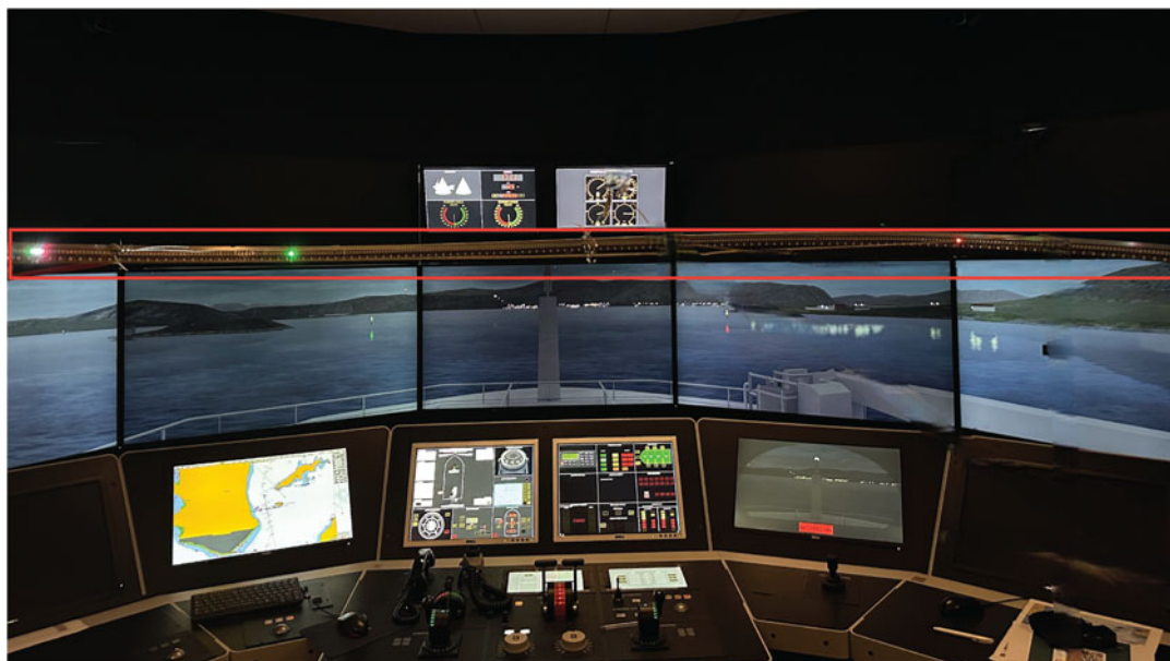
Figure 5. mHUD (lights highlighted with red frame) installed in the ship bridge simulator over the officer on watch.
