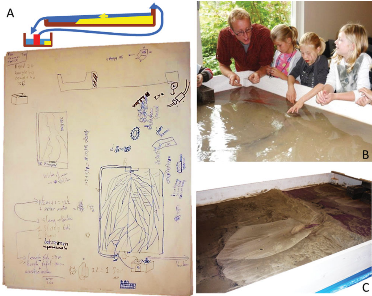
Fig. 3. A set-up of sandbox experiments in Primary School De Klokbeker, Ermelo. A. Example of the design of the sandbox and the hydrological cycle simulated with the pump by pupils. B. Delta experiment, showing explanation by a scientist and impatience to manipulate the experiment in a pupil. C. Dike breach experiment (from right to left), showing a scour hole and splay that pupils compared to real splays in Google Earth.
