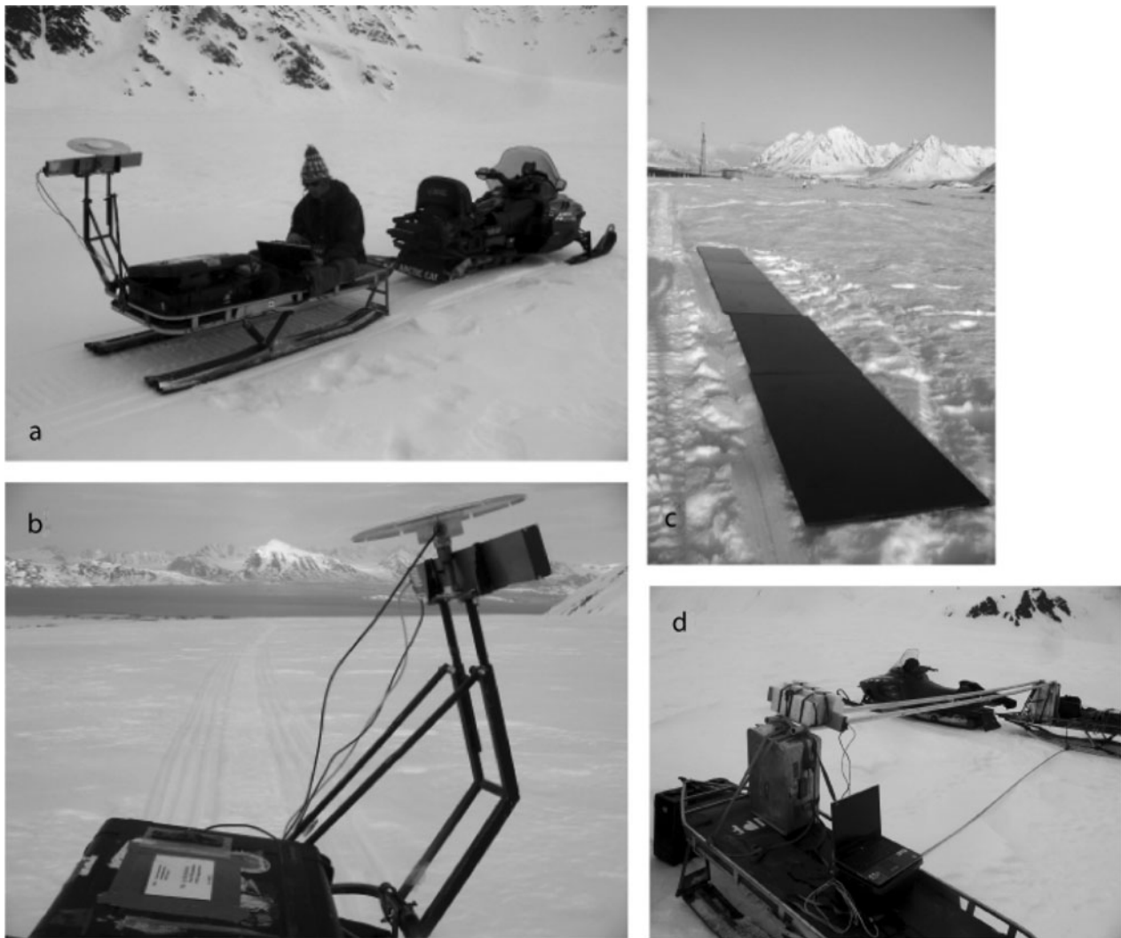
Fig. 1. Pictures of the set-up: (a) general overview of operations; (b) laser and GPS set-up; (c) wooden plate used for the calibration; and (d) laser measurements made on poles.
