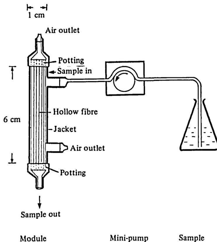
Fig. 1. A schematic diagram of filtration treatment.
