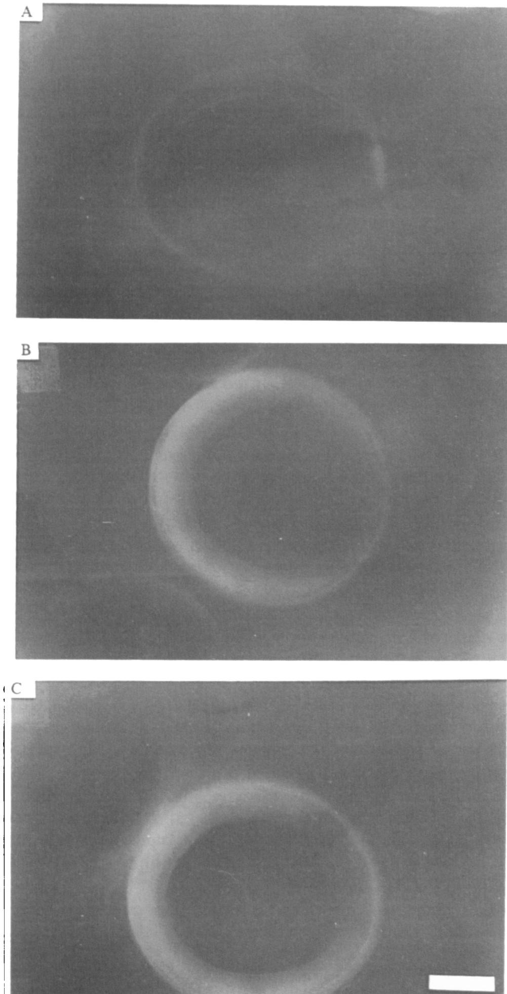
**Fig. 5.** Microscopic feature of FITC-LPS adsorbed EHF membrane. A, untreated control; B, FITC-LPS (20 ml) loaded; C, FITC-LPS (30 mL) loaded. A bar indicates 100  $\mu\text{m}$ .
