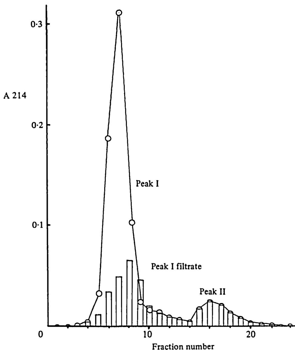
Fig. 2. Chromatographic profile of LPS sonicated on a column of Sephadex G-75 and filtration profile with a membrane.  $\circ$ , Sonicated for 1 min;  $\square$ , filtered with a membrane.
