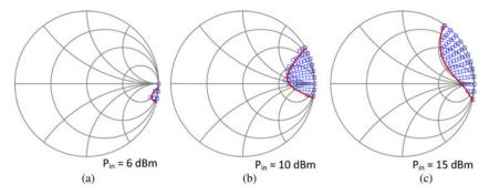
Fig. 3. Instability boundaries, showing also the points fulfilling  $\text{Re}(Y_{To}) < 0$  and  $|\text{Im}(Y_{To})| \le 10^{-3} \,\Omega^{-1}$ . (a) For  $P_{in} = 6$  dBm. (b) For  $P_{in} = 10$  dBm. (d) For  $P_{in} = 15$  dBm.
