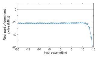
Fig. 11. Pole-zero identification of the matched amplifier (terminated in 50  $\Omega$ ), with a stabilization resistor  $R_s=82~\Omega$ . This analysis complements the one based on the admittance diagrams in Fig. 10. Combining the results of the two analyses, it is predicted that the amplifier will be unconditionally stable under mismatch effects for  $R_s<82~\Omega$ .
