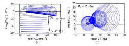
**Fig. 2.** Graphical method to obtain initial values, using the total admittance function. (a) Results in the case of an incommensurable frequency f, sweeping in f,  $ρ_o$ , and  $φ_o$  at the constant input power  $P_{in} = 10$  dBm. No instability boundary can exist within the unit Smith chart. (b) Results in the case of a subharmonic frequency  $f_{in}/2$  and  $P_{in} = 10$  dBm, sweeping  $φ_{in}$ ,  $ρ_o$ , and  $φ_o$ . There should be an instability boundary inside the unit Smith chart.
