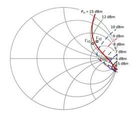
**Fig. 4.** Evolution of the flip locus obtained with (3) versus  $P_{in}$ . The loci only cross the Smith chart in a certain  $P_{in}$  interval. The two reflection-coefficient points ( $\Gamma_{t1}$  and  $\Gamma_{t2}$ ) at both sides of the boundary corresponding to  $P_{in} = 15$  dBm (used for the validation of the method) are indicated.
