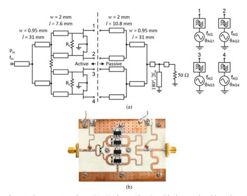
Fig. 8. PA based on four active devices, operating at  $f_{in} = 1.5$  GHz. (a) Schematic. The AGs used for the potential-instability analysis and operating at the frequency  $f_{AG}$ , are also shown. Their phases,  $\phi_{AG_3}$ ,  $\phi_{AG_2}$ ,  $\phi_{AG_3}$ , and  $\phi_{AG_4}$  depend on the particular odd mode to be analyzed, as described in the main text. (b) Photograph.
