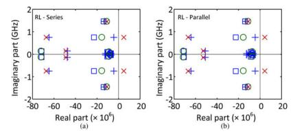
Fig. 5. Validation of the flip locus corresponding to  $P_{in} = 15$  dBm with two different implementations of  $\Gamma_{t1}$  and  $\Gamma_{t2}$  in Fig. 3. (a) RL-series implementation. Poles of the  $\Gamma_{t1}$  ( $\Gamma_{t2}$ ) load are represented with "+" ("x"). (b) RL-parallel implementation. Poles of the  $\Gamma_{t1}$  ( $\Gamma_{t2}$ ) load are represented with "+" ("x").
