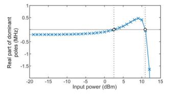
**Fig. 9.** Stability analysis of the PA terminated in a standard 50  $\Omega$  load, with a stabilization resistor  $R_s = 100 \Omega$ , connected as shown in Fig. 8. The real part of the dominant poles has been represented versus  $P_{in}$ . The frequency f of these poles is incommensurable with the input frequency  $f_{in}$ . The PA is unstable in the interval comprised between  $P_{in1} = 2.55$  dBm and  $P_{in2} = 10.9$  dBm.
