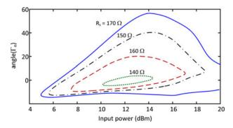
**Fig. 6.** Calculation of the unstable  $P_{in}$  interval using the locus in (4). The limits of this interval correspond to the edge points of the locus. The calculation has been performed for different values of the stabilization resistor  $R_s$ .
