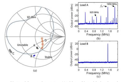
Fig. 14. Experimental measurement of the PA with four active devices in Fig. 8. (a) Validation of the instability boundary under incommnesurable oscillations in the odd mode  $\begin{bmatrix} 1 & 1 & 1 \end{bmatrix}^T$ , corresponding to the input power  $P_{in} = 10$  dBm. (b) Unstable behavior for the experimental load A. (c) Stable behavior for the experimental load B.
