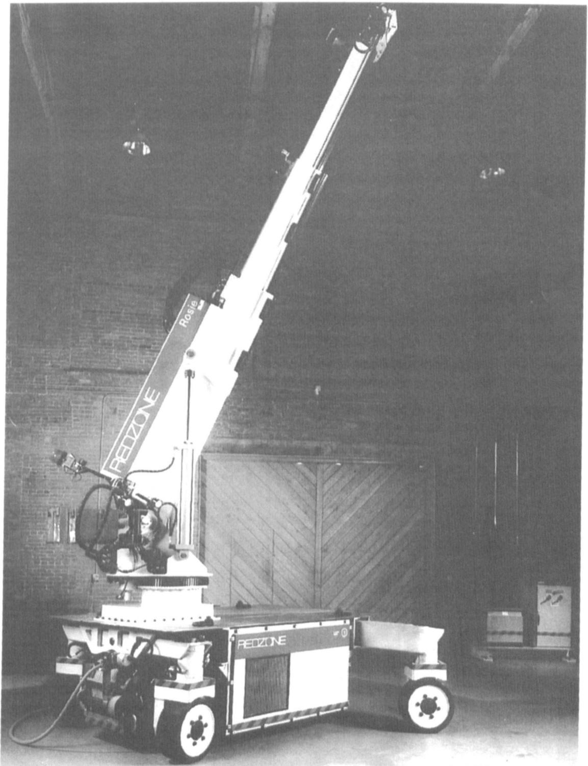
**Figure 2.** "Rosie" broke up high-density concrete in an hour compared to several days for workers using a jackhammer. Department of Energy photo.
