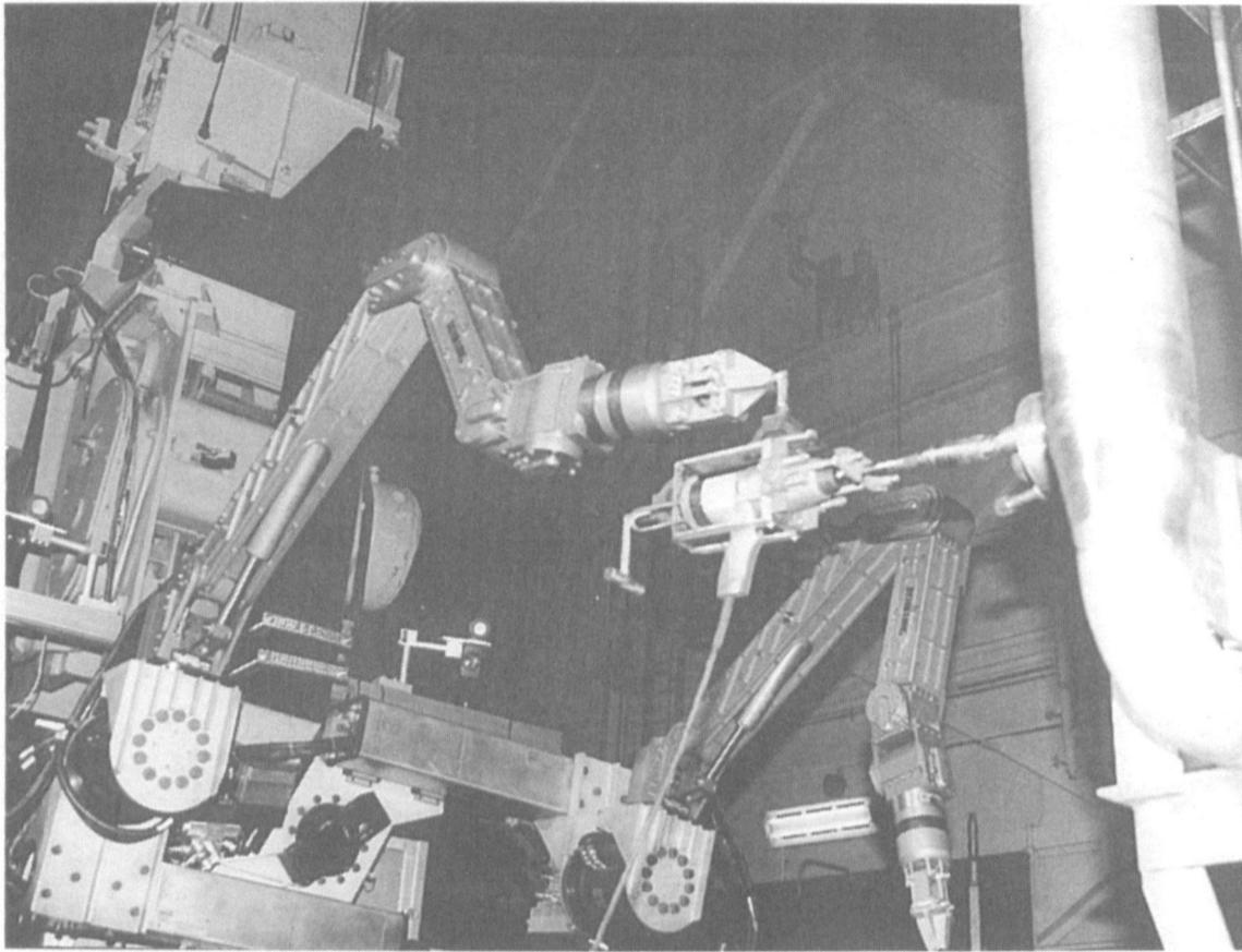
**Figure 3.** The Dual-Arm Work Platform can manipulate a variety of tools and its remote operation removes workers from high radiation environments. Department of Energy photo.
