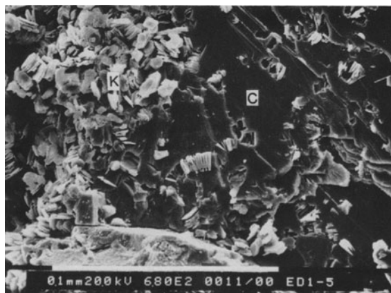
Figure 4. SEM photomicrograph showing calcite (C) engulfing kaolinite (K) pore fill. Eddystone #1, 886.01 m.
