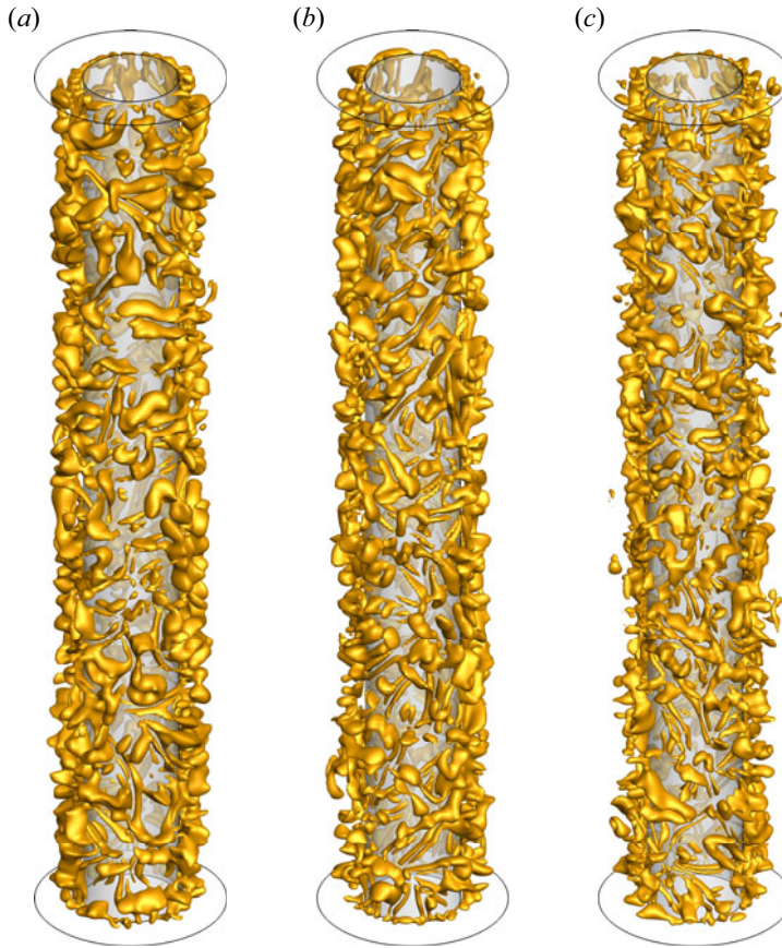
Figure 26. The 3-D vortical structures for (a) V_E = 7000 ( Q = 100 ), (b) V_E = 8000 ( Q = 150 ) and (c) V_E = 10000 ( Q = 300 ).
