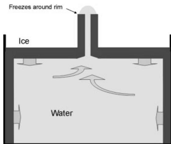
Fig. 4. The Bally–Dorsey model for ice-spike formation. Ice spikes grow as the solidification process forces water up through an ice tube, where it freezes and lengthens the tube. As described in the text, this model can explain why ice spikes form preferentially in pure water and in the presence of air-flow.
