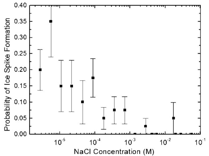
Fig. 3. Probability of ice-spike formation as a function of the solution concentration of table salt in deionized water.
