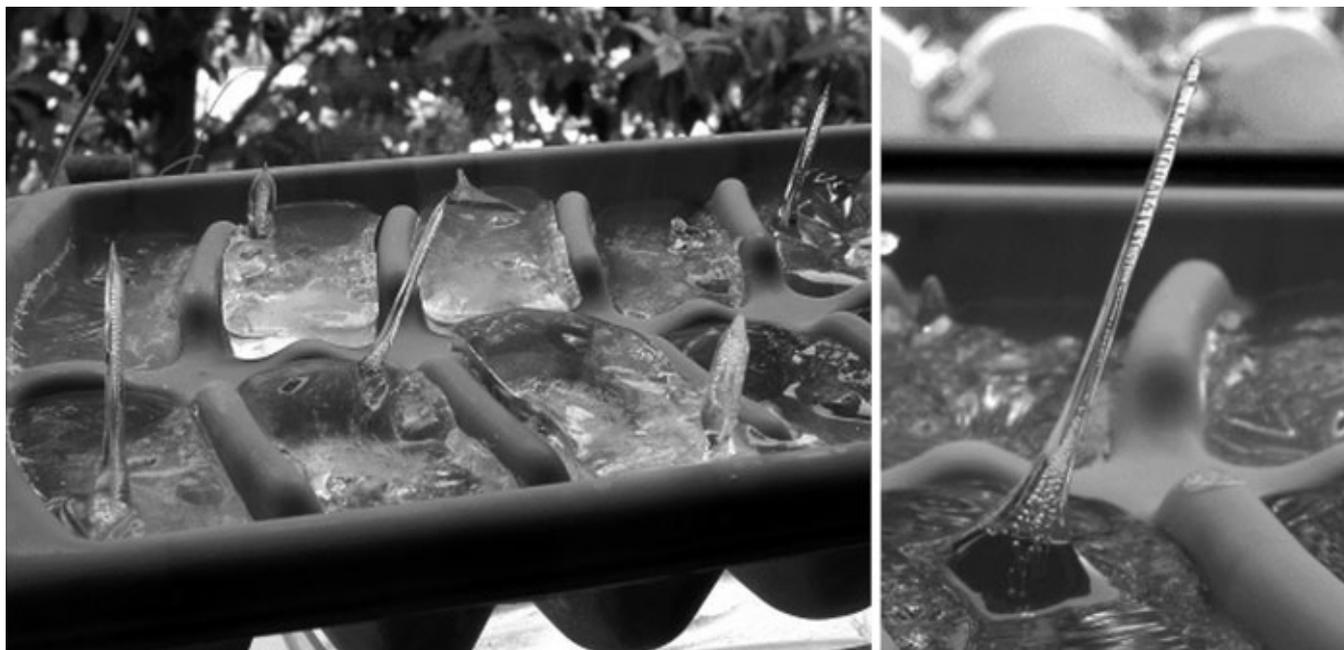
Fig. 1. A number of ice spikes grown in an ordinary plastic ice-cube tray using distilled water. Note the spikes grow at many different positions and angles and to various heights up to  $\approx 50$  mm.
