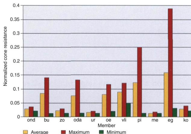
Fig. 6. Values of normalized cone resistance for every stratigraphic member. Average, maximum and minimum values from cone penetration tests. ond: Onderdijke; bu: Buisputten; zo: Zomergem; oda: Onderdale; ur: Urssel; oe: Oedelem; vli: Vlierzele; pi: Pittem; me: Merelbeke; eg: Egem; ko: Kortemark.
