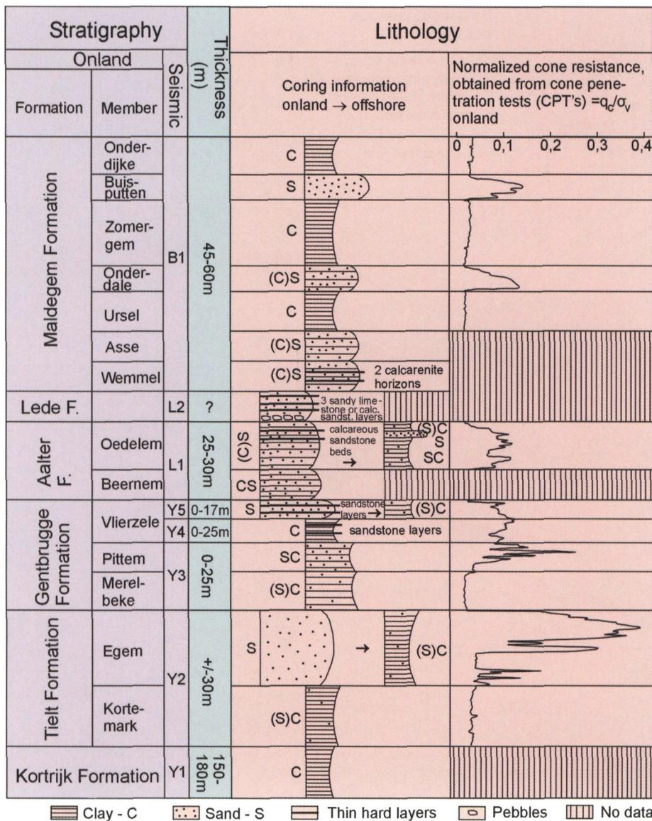
Fig. 5. Lithostratigraphy of Eocene deposits. Synthetic logs compiled from onland to offshore coring information (left) and onland typical normalized cone resistance parameter profiles (right). On a depth basis, correlation has been realised between coring and seismo-stratigraphic information, and coring and cone resistance information.
