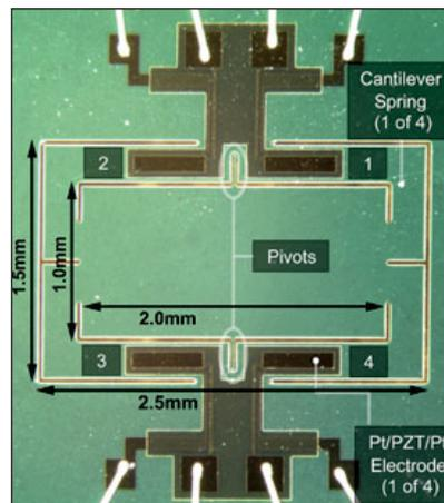
A photograph of the biologically inspired microphone taken under a microscope, providing a top-side view. The tiny structure rotates and flaps about the pivots (labeled), producing an electric potential across the electrodes (labeled). Credit: N.Hall/UT Austin.
