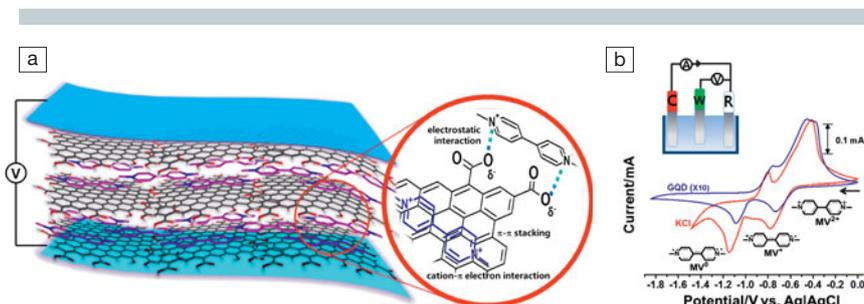
(a) Illustration of an electrolyte-free flexible electrochromic device of  $MV^{2+}$  graphene quantum dots (GQDs). (b) Cyclic voltammogram of 5 mM  $MV^{2+}$  at an indium-tin-oxide electrode in an aqueous solution containing 8 mg mL<sup>-1</sup> GQD (blue line) and 0.1 M KCl (red line) at a scan rate of 100 mVs<sup>-1</sup>. Inset: A depiction of a three-electrode cell composed of a working electrode (W), a counter electrode (C), and a reference electrode (R). Reproduced with permission.
