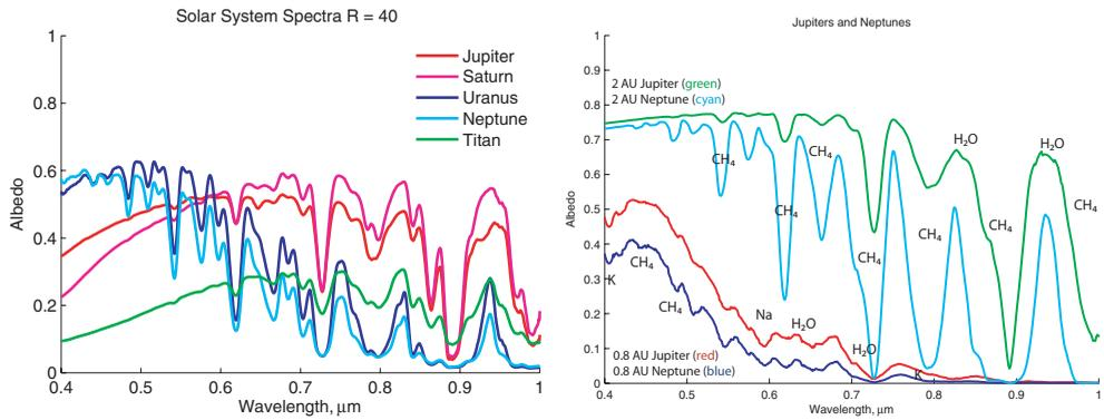
**Figure 1.** Right: Albedo of some planets in the Solar System (Karkoschka 1994) smoothed to SPICES resolution,  $R = 40$ . Left: Albedo of model Jupiter and Neptune planets from Cahoy *et al.* (2010) at separations of 0.8 AU (red and dark blue, too warm for clouds) and 2 AU (green and cyan, just cold enough for water clouds) smoothed to SPICES resolution,  $R = 40$ .
