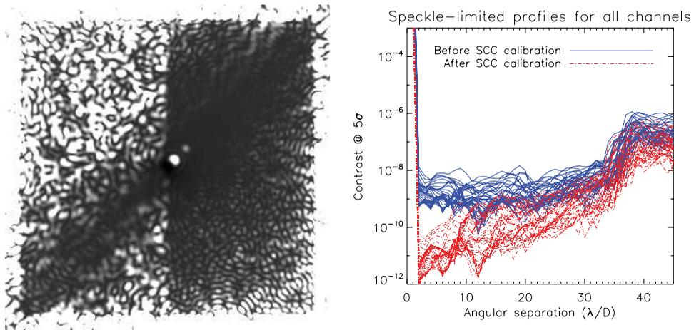
**Figure 2.** Left: simulated images of SPICES in one spectral channel ( $\lambda = 675\text{nm}$ ) showing the  $64 \times 64\lambda/D$  corrected field of view where two fake planets at  $10^{-8}$  and  $10^{-9}$  contrast were added. Right: Corresponding 5-sigma contrast curves of SPICES for all spectral channels, with wavefront control alone (blue) then with an additional speckle calibration technique (red).
