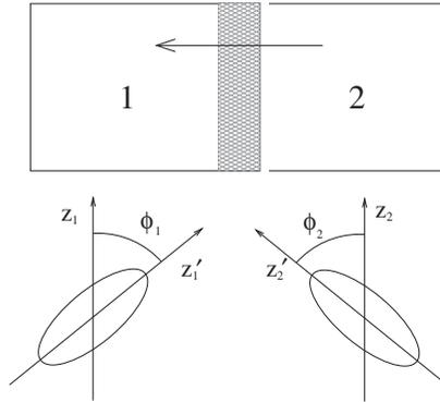
Figure L.1. Schematic representation of a Josephson junction.
