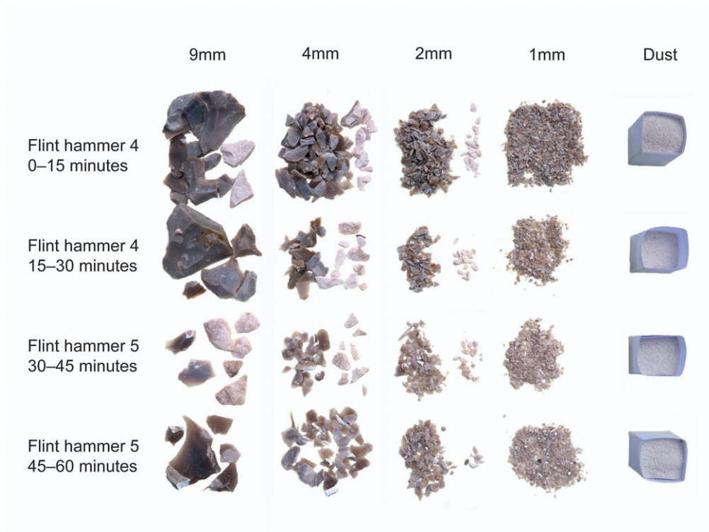
Fig 5. Variations in residues by sieve mesh size and time using flint hammers 4 and 5 to peck dress one surface of the block in a period lasting sixty minutes. The blue boxes represent 1cu inch (16.38cu cm). Photograph: author.
