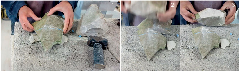
Fig 2. Point loading: 1) showing block resting on sarsen supports; 2) the blow delivered; 3) the resulting squared fracture. Photographs: author.
