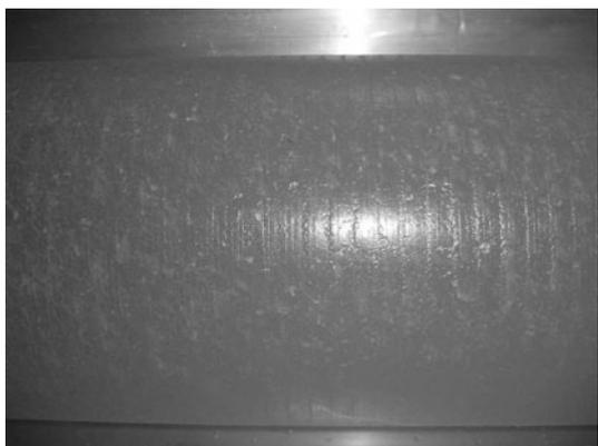
**Fig. 7.** Core cut with sharp corner cutters.
