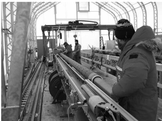
**Fig. 9.** Screen-cleaning system being used manually.
