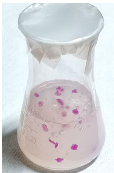
Fig. 6. Gelatinous Mn–As-bearing substance with aggregates of krautite crystals. The gel was prepared by mixing two solutions (see Buckley et al. , 1990) about 6 weeks before the photograph was taken.
