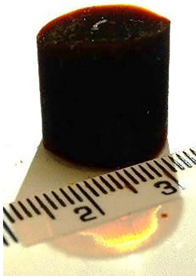
Figure 5. Fe(III)-based aerogel monolith using iron(III) chloride hexahydrate and TO.
