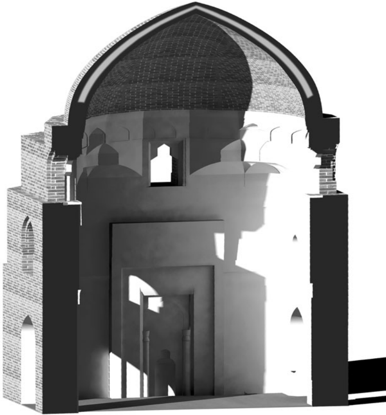
Figure 6. Dome chamber, 3d section view
