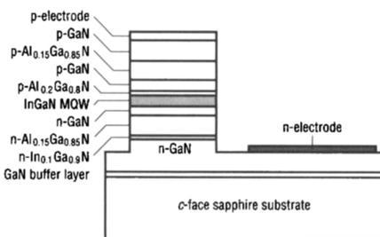
The structure of the InGaN MQW laser diode.
