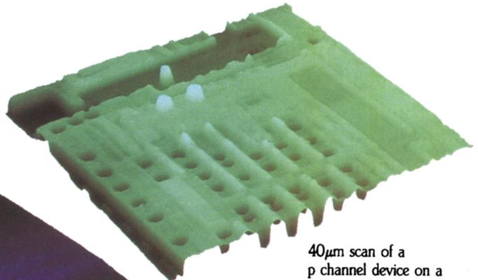
40 $\mu$ m scan of a p channel device on a semiconductor wafer
