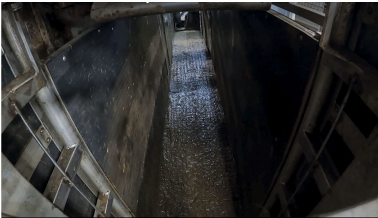
Figure 1. Photographic view from the entrance of the rump pusher (RP) towards the stun box. Both entrance and exit gates of the RP are open with the RP in the upright position.
