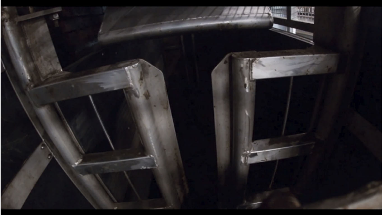
Figure 2. Photographic view from the entrance of the rump pusher (RP) towards the stun box. Both entrance and exit gates of the RP are closed with the RP in the upright position.
