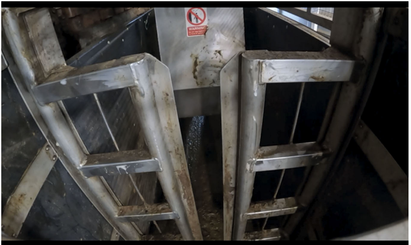
Figure 3. Photographic view from the entrance of the rump pusher (RP) towards the stun box. The entrance gate is closed, and the RP is in the downwards position. From this position the pusher would move forward towards the stun box.
