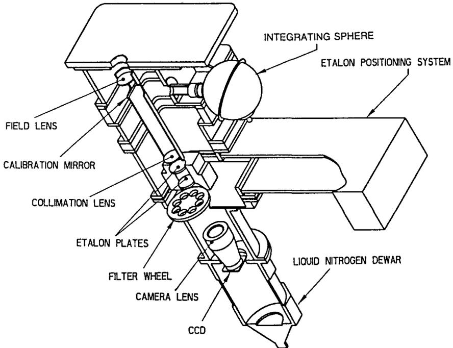
Figure 1. A schematic of the GFPI optical path.
