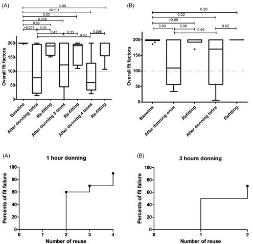
**Fig. 2.** Overall fit factors of the participants at baseline and after repetitive donning/doffing. (A) Results of 1-hour-donning. (B) Results of 3 hours donning. Boxes represent the median and interquartile range [IQR]. Whiskers indicate the upper and lower adjacent values (within  $1.5 \times IQR$ ), and isolated dots are outlier data points.
