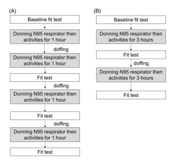
Fig. 1. Schematic flow chart of the fit test.
