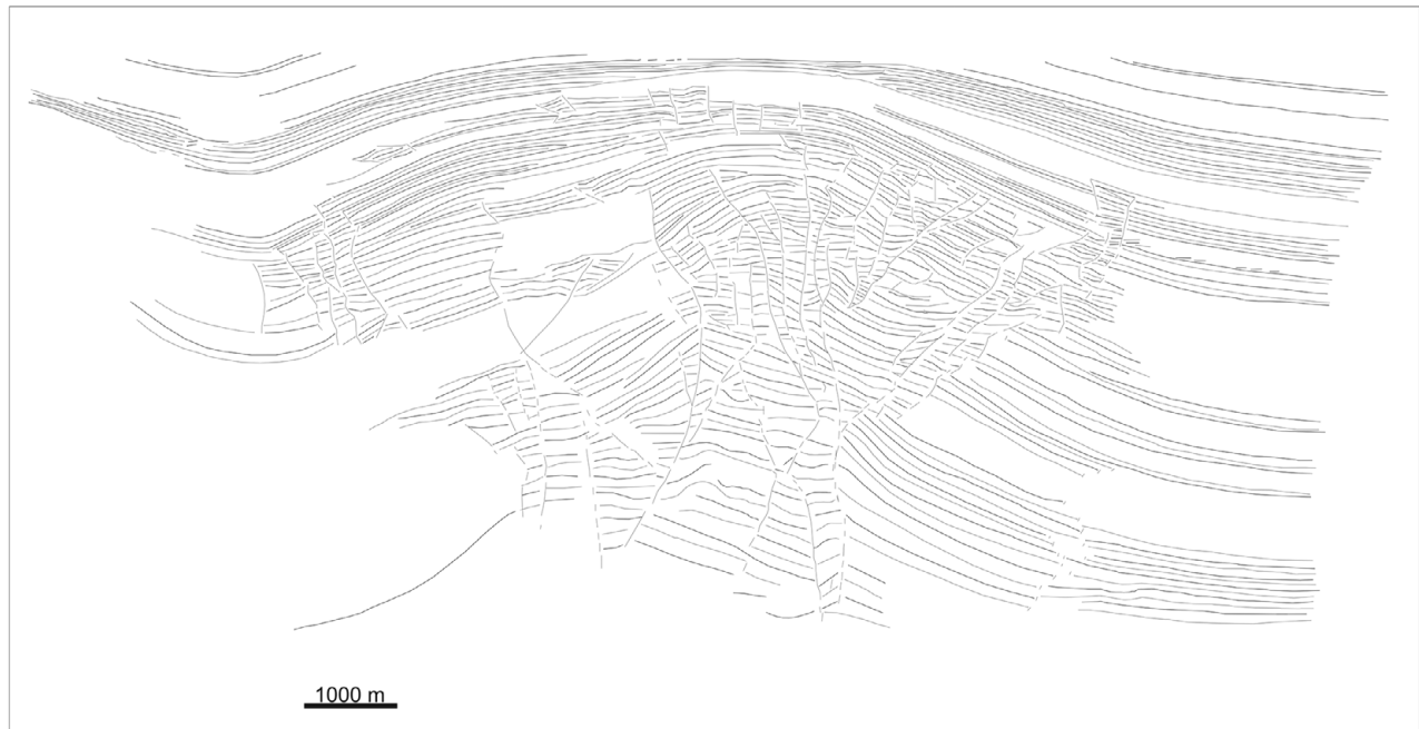
Figure 1.18 (b) Line drawing of the NNE–SSW striking reflection seismic profile through the Elk Hills anticline, Southern San Joaquin Basin, showing a positive flower structure (Nemčok and Schamel, 2000).
