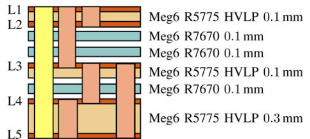
Fig. 14. Multilayer stack of the frontend assembly.
