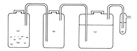
Fig 1. Carbon dioxide absorption train: (a) dry-ice snow in 50L carbouy; (b) gas-diffusion volume; (c) 60L 8M KOH in 100L carbouy; (d) absorption indicator trap (Ba(OH)<sub>2</sub> solution)
