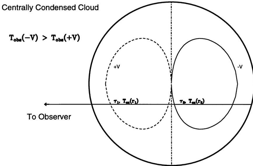
Figure 2. A schematic diagram of a spherical cloud in collapse. This is the case when the infall velocity increases toward cloud center. The oval shaped lines are tracks of constant projected velocity. There are two points along a given line of sight with the same projected velocity.
