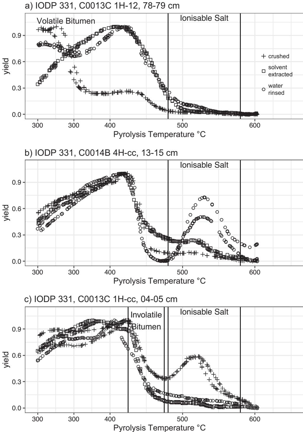
**Figure 2.** Pyrograms of hydrothermally altered volcanic sediment that illustrate the consequences of analytical interferences by (a) IODP 331, C0013C 1H-12, 78–79 cm—effected by bitumen, (b) IODP 331, C0014B 4H-cc, 13–15 cm—affected by ionizable salts, and (c) IODP 331, C0013C 1H-cc, 004–005 cm—sample with a low TOC and effected by bitumen and ionizable salt. Note that the initial stage is isothermal at 300°C, thus 300°C appears successively on the x-axis in the early part of the pyrogram.
