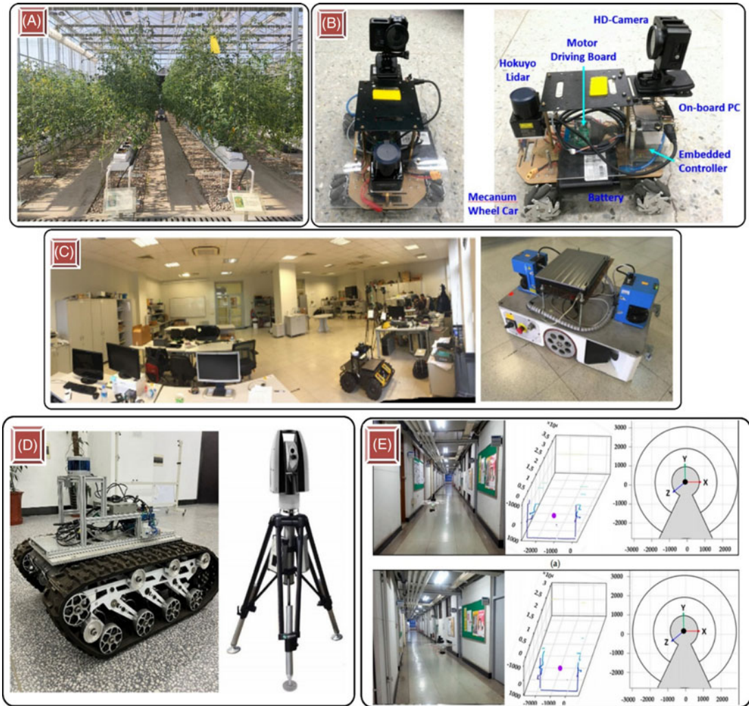
Figure 4. (A) LiDAR-based SLAM system for autonomous robots, taken from ref. [91], copyright frontiers. (B) LiDAR-based robust for pose estimation in clean and perturbed environments [92], copyright MDPI. (C) self-adaptive Monte Carlo Localization algorithm tailored for smart automated guided vehicles position tracking, and kidnapping scenarios, taken from ref. [93], copyright elsevier. (D) LiDAR localization method leveraging multi-sensing data from IMU, odometry, and 3D LiDAR for complex indoor spaces, taken from ref. [94], copyright MDPI. (E) LiDAR and IMU integration for UAV indoor navigation, taken from ref. [95], copyright MDPI.
