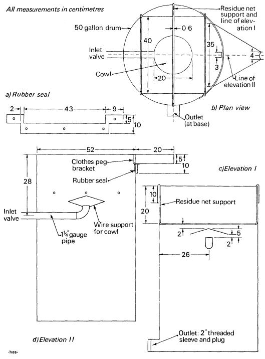
Fig. 1. Blueprint of the Sīrāf flotation unit
