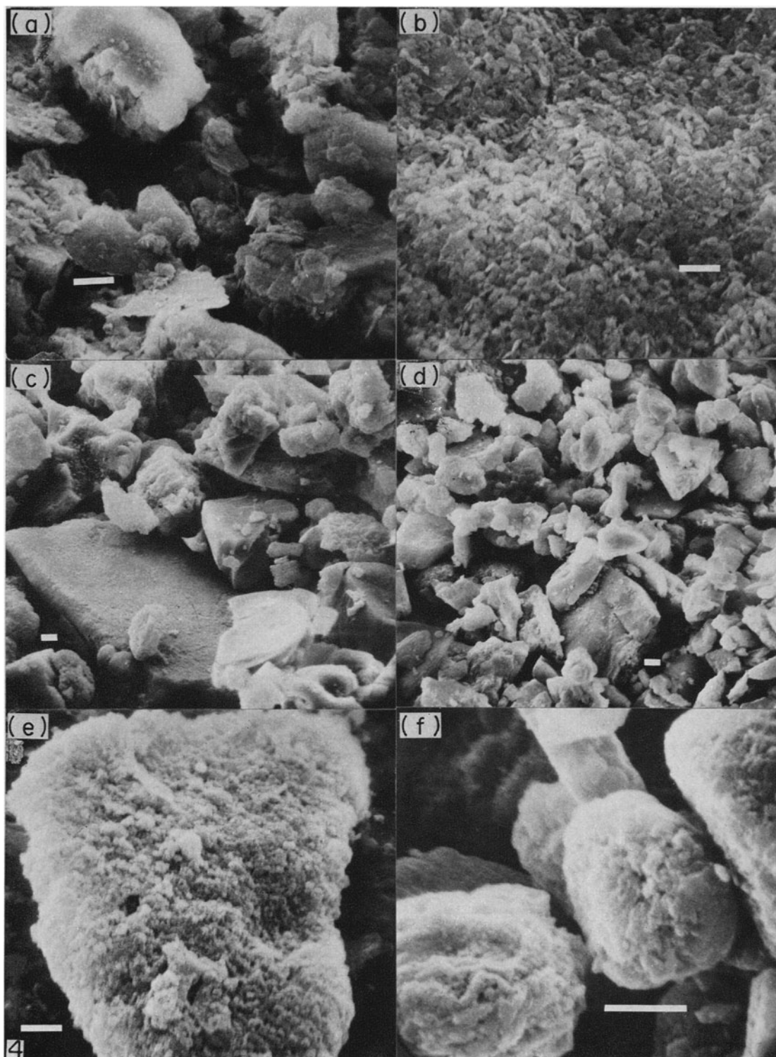
Fig. 4. Scanning electron micrographs: (a) kaolinite sample 1a (Twiggs, coarse), and (b) kaolinite sample 2a (Twiggs, fine), both easily magnetically separated; (c) the coarse (\text{Ti,Fe})\text{O}_2 isolate (rich in rutile, Fig. 2), from kaolinite sample 1a, after extensive heavy liquid treatments and separation by sedimentation in water; (d) the fine isolate (richer in anatase), resulting from the same water separation; (e) a mica particle loaded with fine anatase in the (\text{Ti,Fe})\text{O}_2 isolate from kaolinite sample 3b; (f) a (\text{Ti,Fe})\text{O}_2 isolate (from kaolinite sample 1a), at higher magnification, showing roughness which possibly resulted from hot NaOH etching before the \text{H}_2\text{TiF}_6 treatment. The bar indicates 2\ \mu\text{m} .
