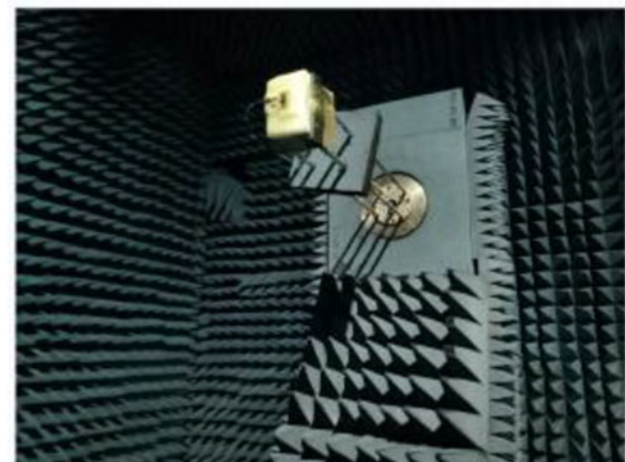
Figure 3. Measurement in an anechoic chamber.
