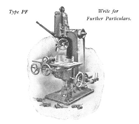
For boring, drilling, and recessing the bosses of propellers, etc.; half lapping the laminations; recessing and drilling the spars, etc.
