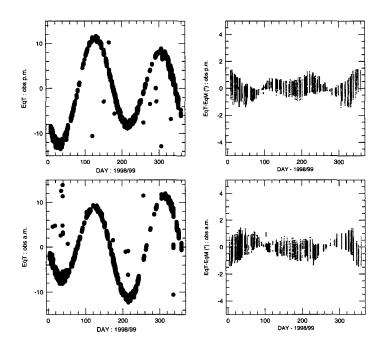
Figure 8. On the left, the Equation of Time as adjusted by the Observatório Nacional eastern and western measurements. On the right, residuals from the adjusted solutions to the standard curve (in arcsec).
