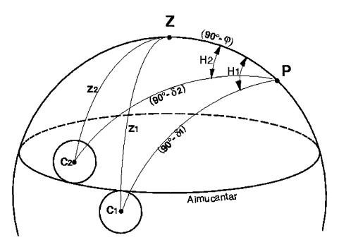
Figure 1. Geometry at solar crossing through an almucantar.
