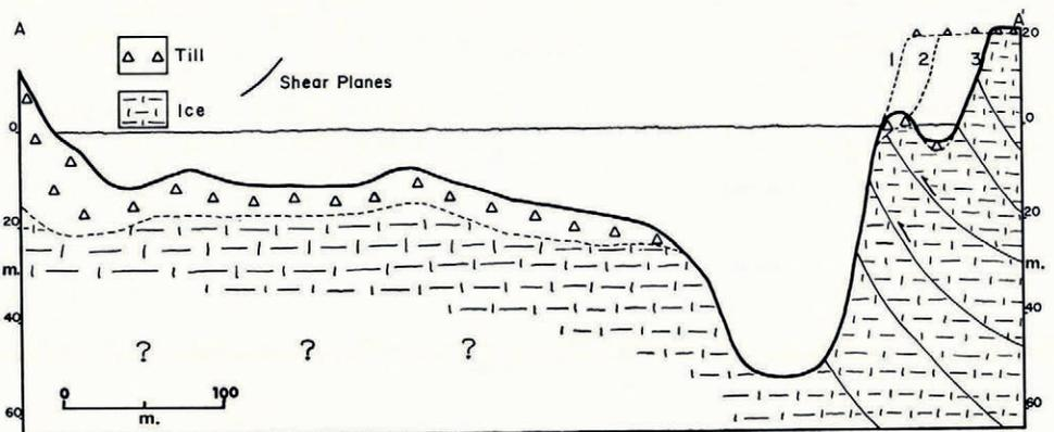
Fig. 4. Idealized cross-section showing successive stages in the formation of "Gull Island" and its relationship to the shear planes. The depression represents the site from which the iceberg emerged. The vertical scale is three times the horizontal scale
