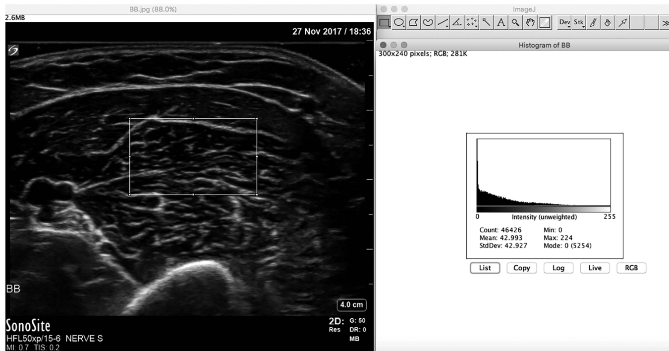
Figure 15: Screenshot of the ImageJ free software program for calculating mean grayscale value from the muscle ultrasound image histogram. The rectangle in the left half of the image denotes the region of interest from which the histogram is captured.
